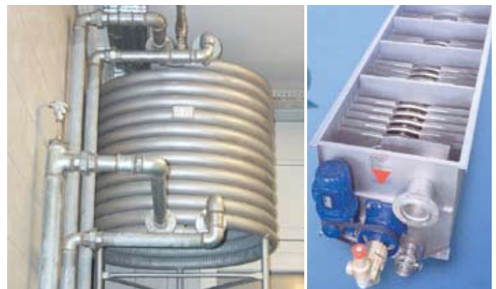
Above, a thermal oil heating system for a tunnel washer and (at right) a water reuse system for a tunnel.
