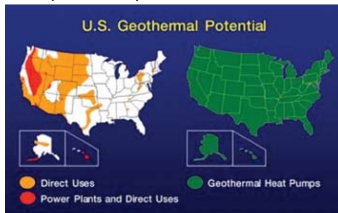
The chart above confirms that much of the Western United States has access to direct use of geothermal power. Geothermal heat pumps can be used nationwide, due to relatively constant shallow ground temperatures.
