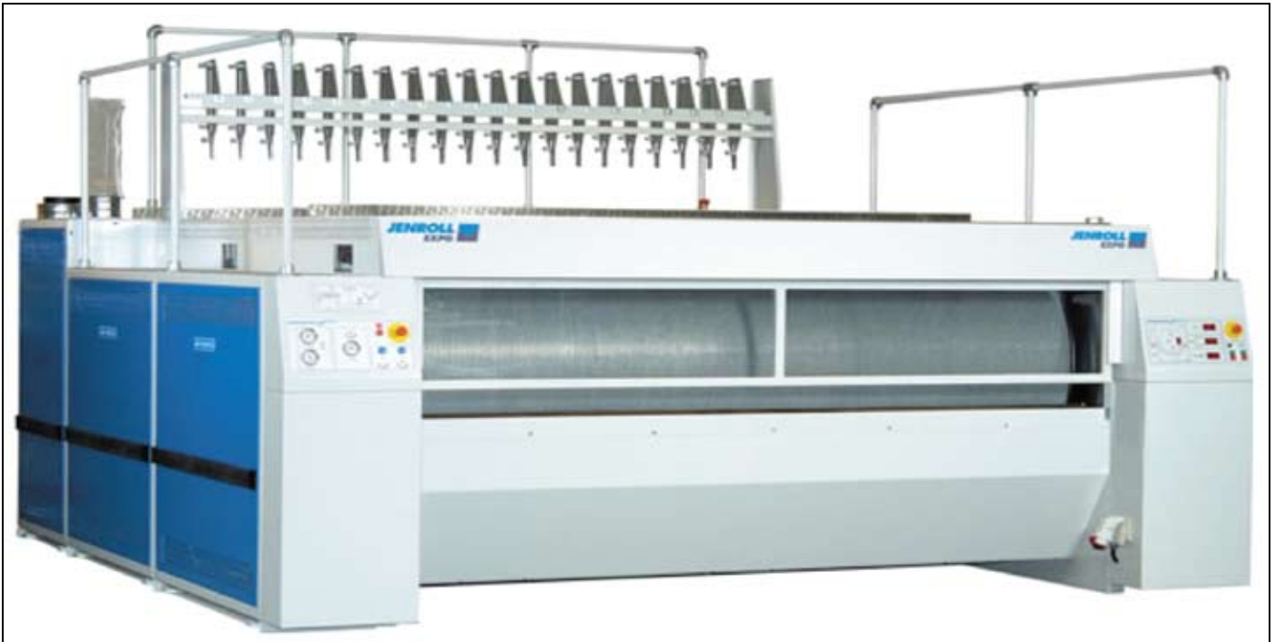
Thermal oil ironing eliminates the inefficiencies of steam leaks with a closed system. The thermal oil also protects against corrosion and thermal oil machines start up easily. Downsides include the fact that every 2-3 years operators must replace the thermal oil these systems use.
