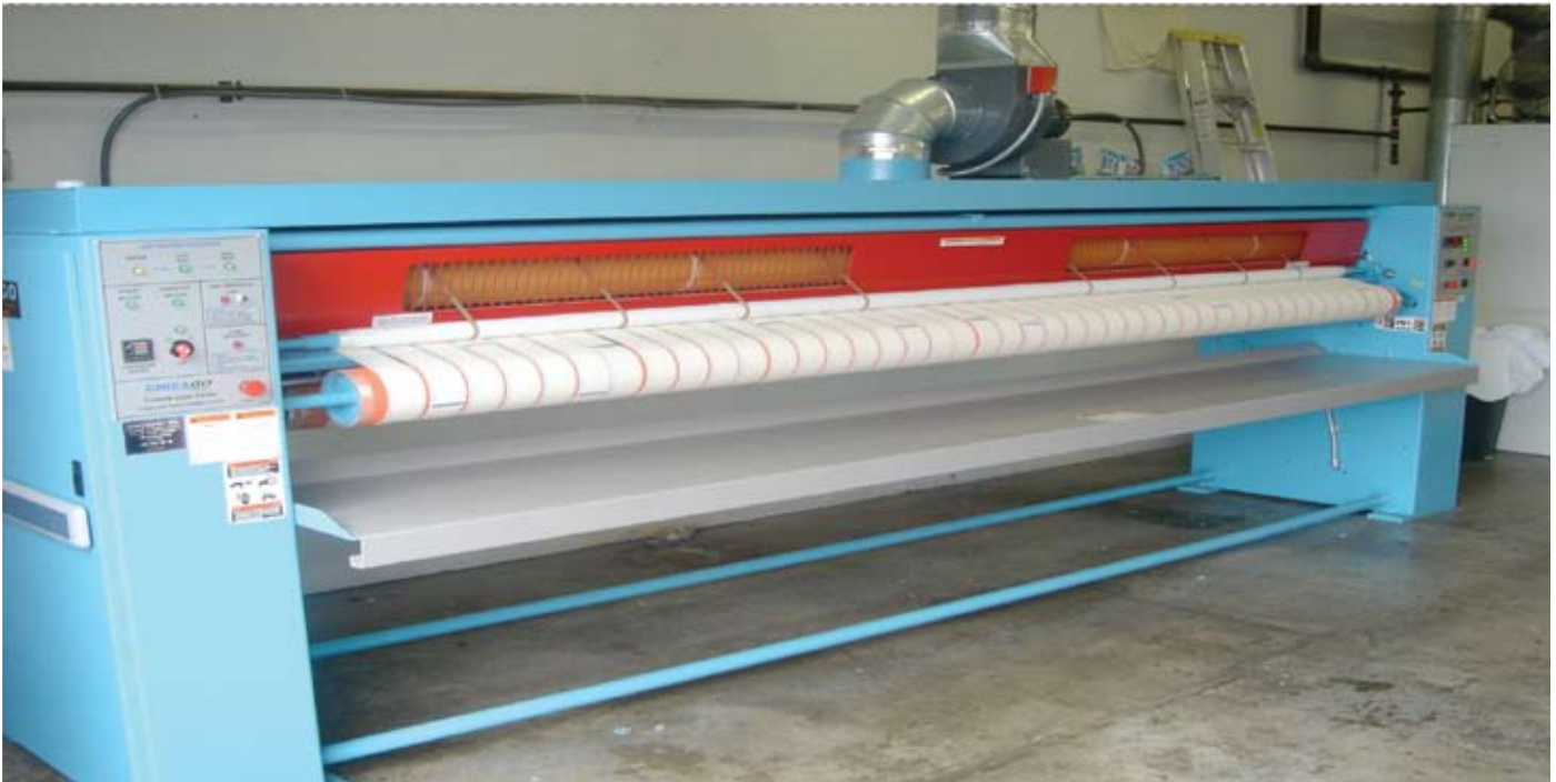
Gas-powered ironers are often smaller, one- or two-roll machines that make sense if floor space or boiler capacity is an issue. They also can run independently from other laundry machinery in the plant and are relatively easy to hook up and operate.
