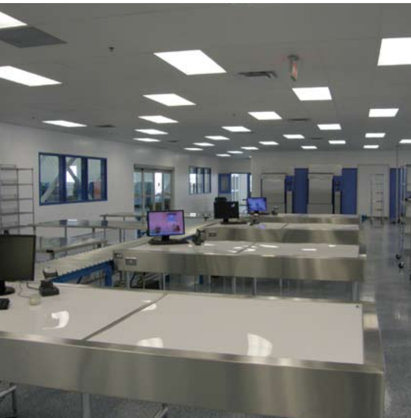
Light tables equipped with computer monitors are used for inspecting garments in the OR packroom. Conveyor equipment is visible to the left of the photo.
