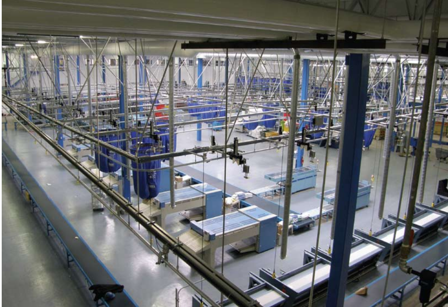
Small-piece folders, conveyors and overhead slings in the plant's finishing department. The author applauds CEO Rocco Romeo's ability to "think outside the box" by planning a facility that could process healthcare and high-end hospitality linens, plus a sterilization area for OR packs and a mat cell for laundering walk-off mats.
