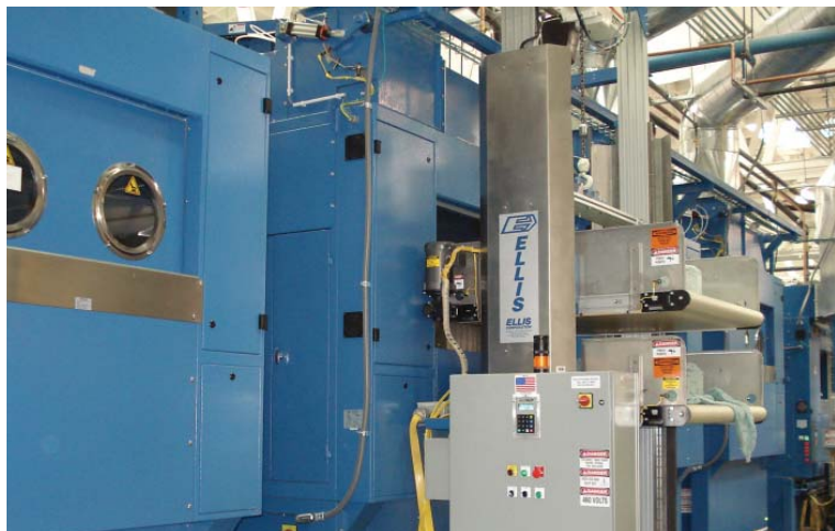
Automating a wash aisle helps reduce the number of carts moving through the plant by hand. With fewer 'touches' by employees, throughput improves.
