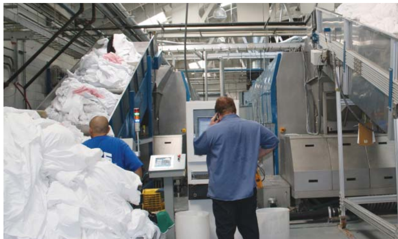
Advances in soil-sorting technology, including high-tech conveyors like the one shown above, increase efficiency by ensuring accurate weights so the proper amounts of water and chemicals are applied to clean the textiles.
