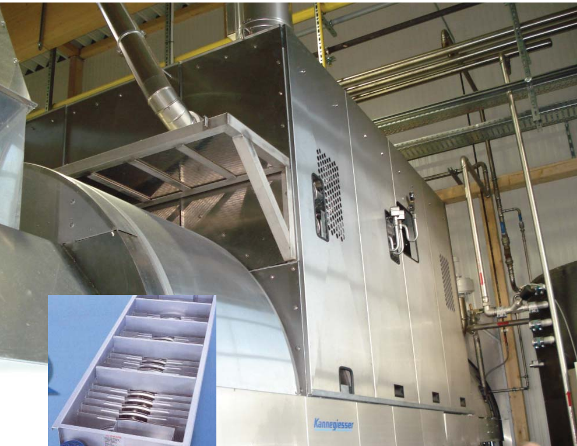
Hot water reuse systems for tunnel washers, like the one at left, are part of a technological trend in Europe driven by costs and regulatory pressures that are encouraging laundry operators to ditch steam boilers and heat water by various other means.
